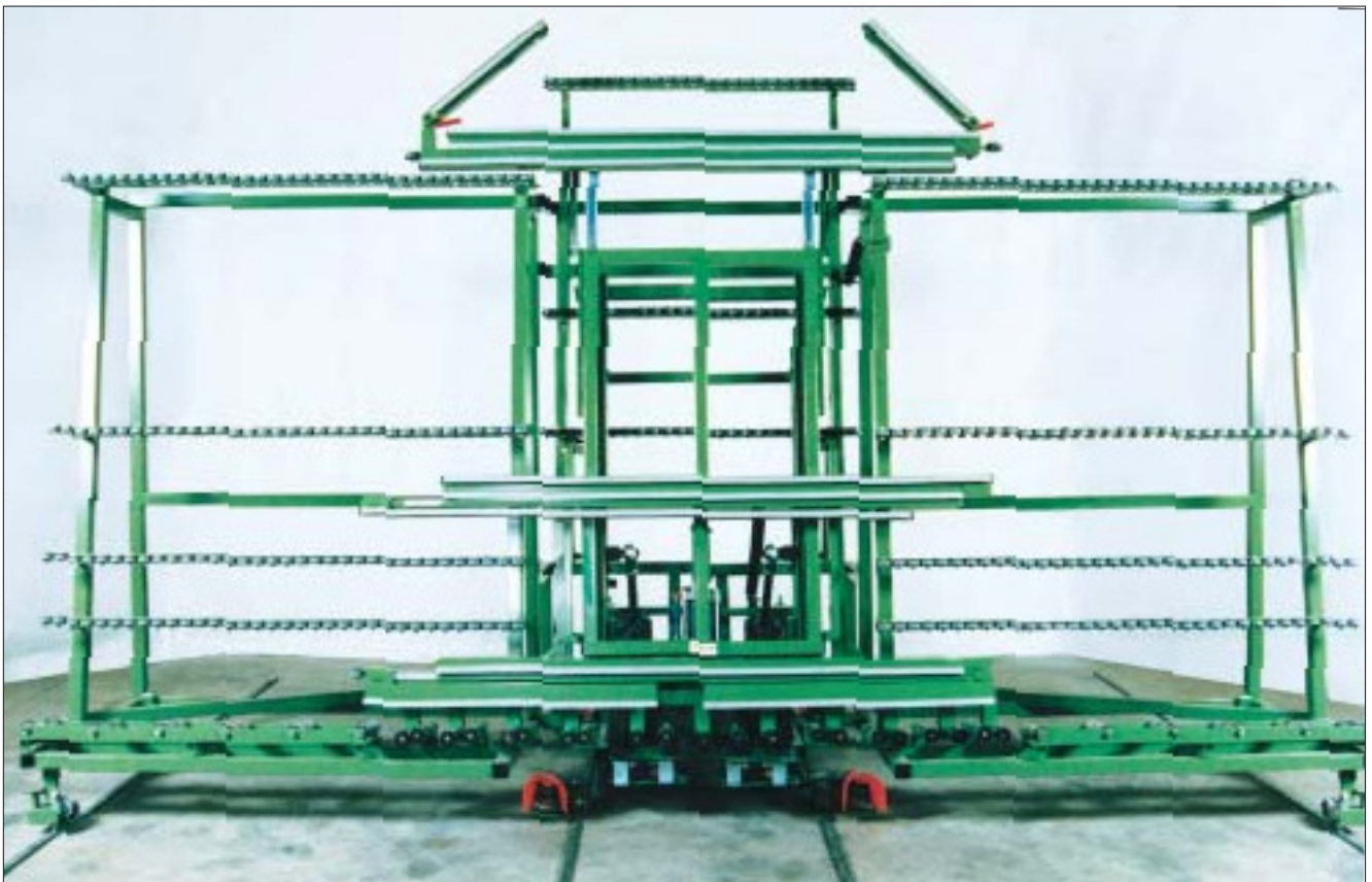
Transfer roller conveyer with movement feature RU-RGAF45/20/2ÜE with retracted table RU-MKSEA-1,4.
