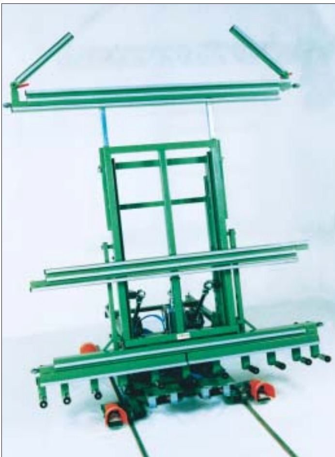
Assembly turn-tilt table in transfer position for simple transfer (without retraction).
