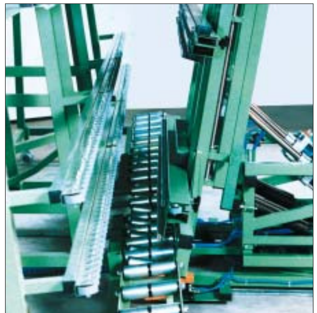
Assembly turn-tilt table in transfer position for simple transfer (without retraction).
